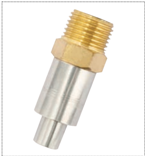
NO 1069 Wet feeding nipple drinker 1/2" brass thread and stainless steel body Hex 21, pipe \Phi 21, pin \Phi 12*15 mm Bowl type, For weaners, fatteners, finishers
