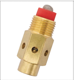
NO 1077 1/2" sprayer drinker Complete brass, Body Hex 22 mm, Length 47 mm, pressure button 17mm, weight: 90g, 4.5 litres/min With holes
