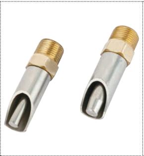
NO 1073 Nipple drinkers 3/8" Brass thread Hex 17mm. Pipe \Phi 16mm, For piglet
