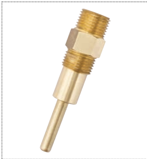
NO 1069 Wet feeding nipple drinker 1/2" brass thread and stainless steel body Hex 21, pipe \Phi 21, pin \Phi 12*15 mm Bowl type, For weaners, fatteners, finishers
